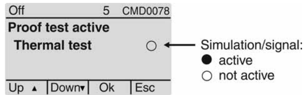
Figure 11: Display indication on local controls
